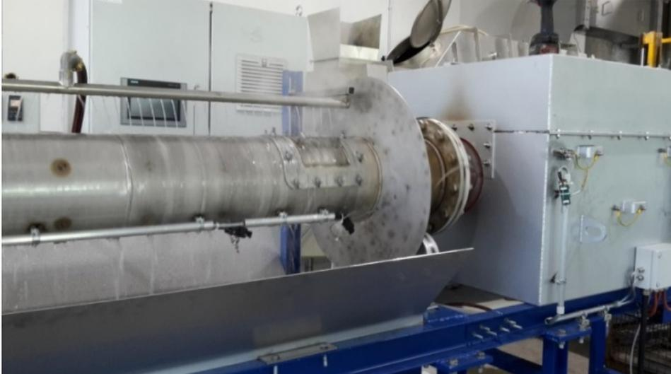
Figure 31: Test plant for continuous solids cooling
