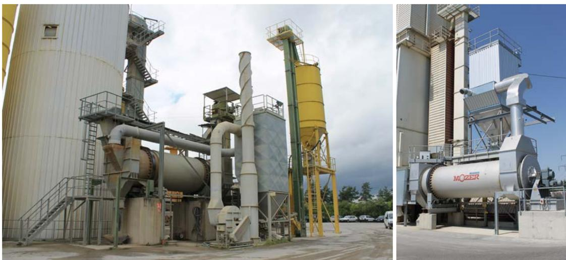
Figure 7: Rotary drums for combined drying and cooling of sand
