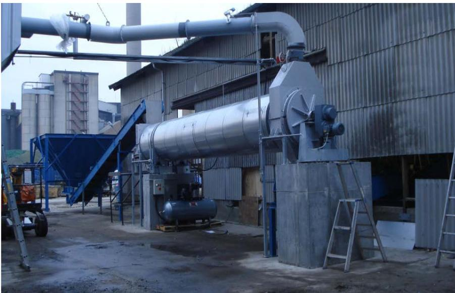
Figure 18: Rotary drying system for recycled glass
