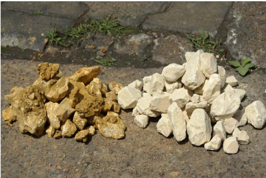
Figure 26: Lime stone samples from before and after the dryer/cleaner TRH
