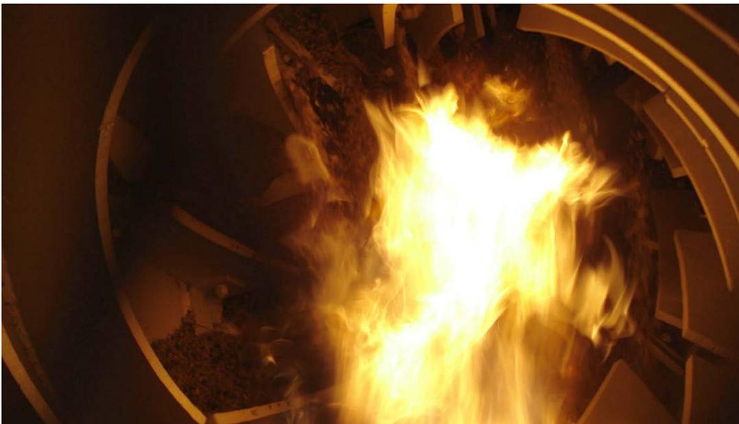
Figure 2: View into a dryer drum with flame in the interior of the drum
