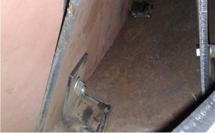
Figure 20: Bolted-on components installed in a drum dryer
