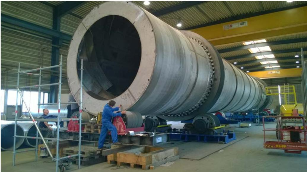
Figure 1: Big rotary drum from stainless steel at the manufacturing hall (4.5 meter in diameter, 35 meter length) for drying of 320 tph fertilizers
