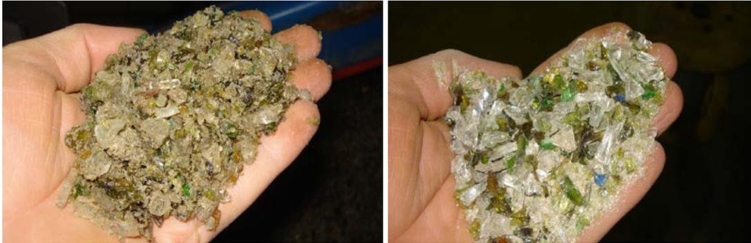
Figure 19: Recycled glass < 10 mm before and after drying
