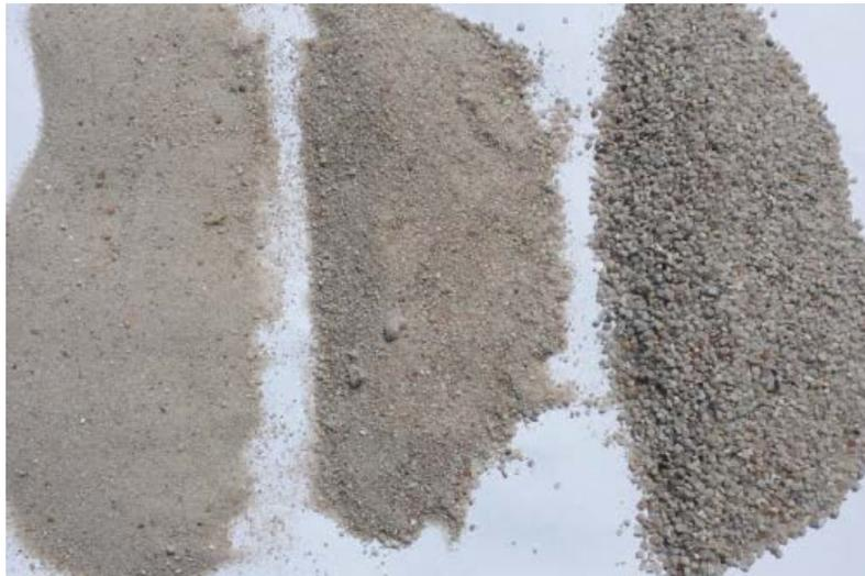
Figure 4: Silica sand with three grain size ranges.
