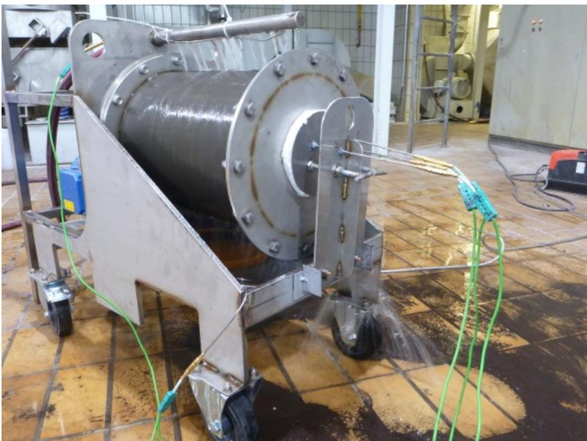
Figure 30: Batch laboratory cooler for determining the properties of bulk materials and heat transfer of real solids
